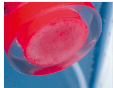
02. Corrosion-protected electrode junctions
